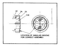
with groove provided. Z1 Engage two springs (9) with pillars provided on closing ring (8).
